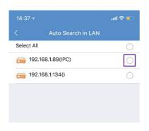
Note: Auto LAN search only works if the http port of the camera remains unchanged (default 80). If the http port has been changed, the camera can only be added manually with its corresponding new port.
